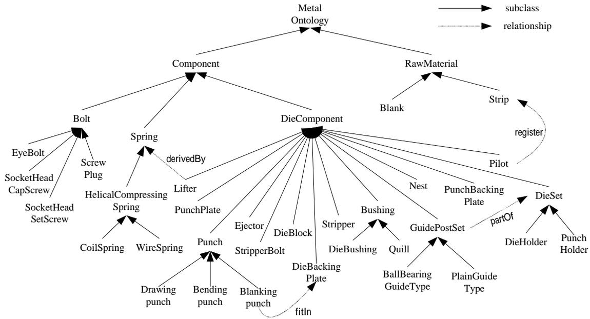
Figure 3. Parts of domain ontology
