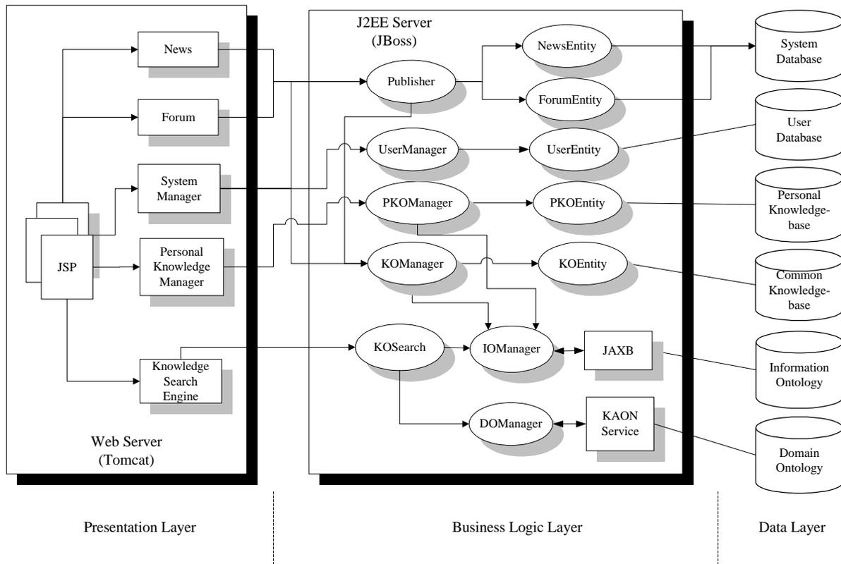
Figure 4. The architecture of ontology-based knowledge management system
