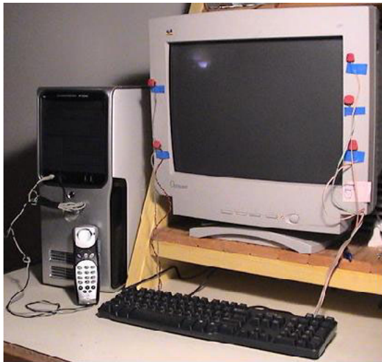
Figure 9: Prototype of flex button with mounted panel keys for input
