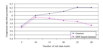
Figure 1. DSP based Gamma vs. Gamma codes.
